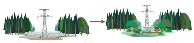
Figure 6. Scheme of a green corridor in transmission lines (Reference: LIFE-ELIA)
